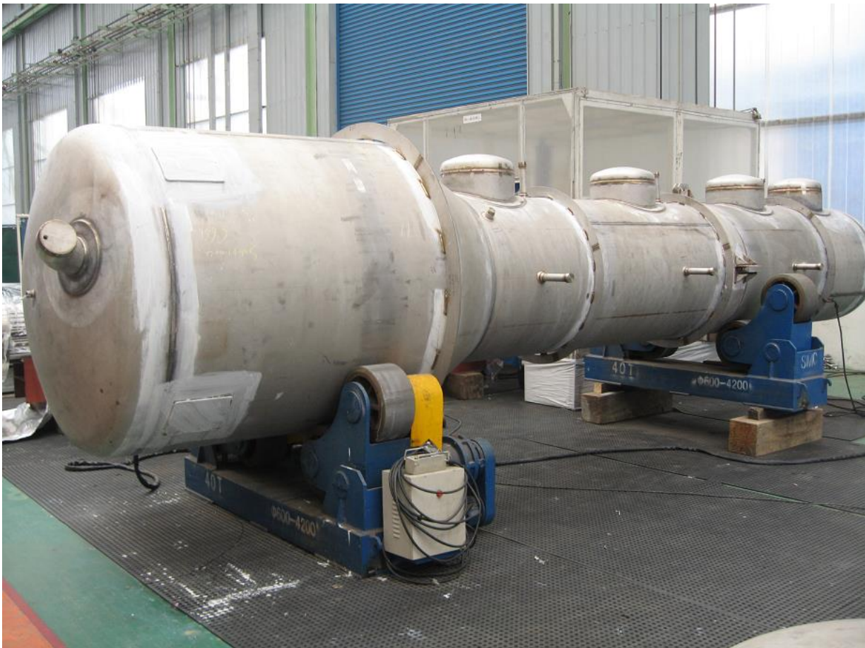
Manufacturing inspection – Check of the manufacturing of the TEP DZ exchangers at Morimatsu (China)
