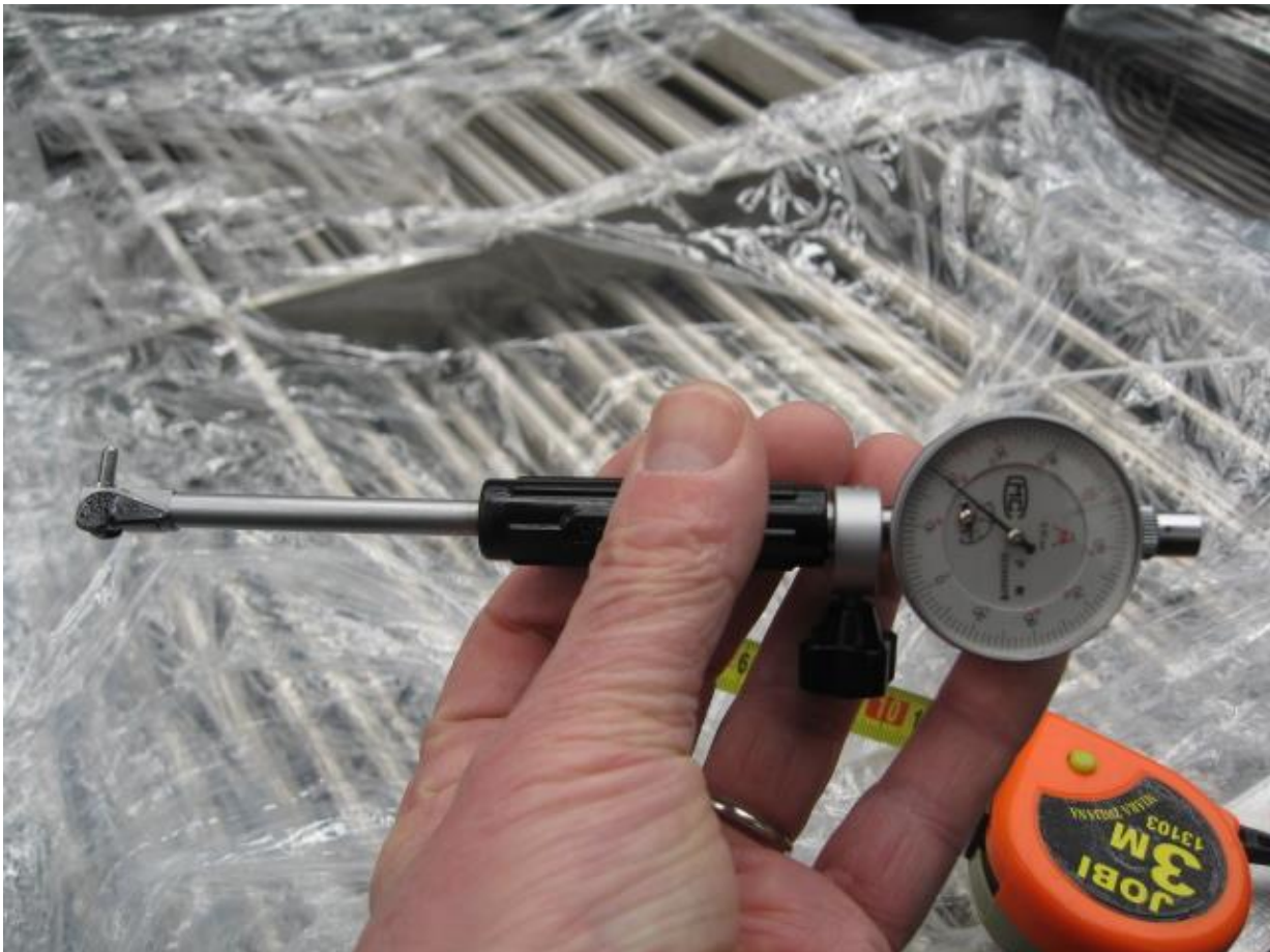
Manufacturing inspection – Check of the tube ID after expansion at Morimatsu (China)
