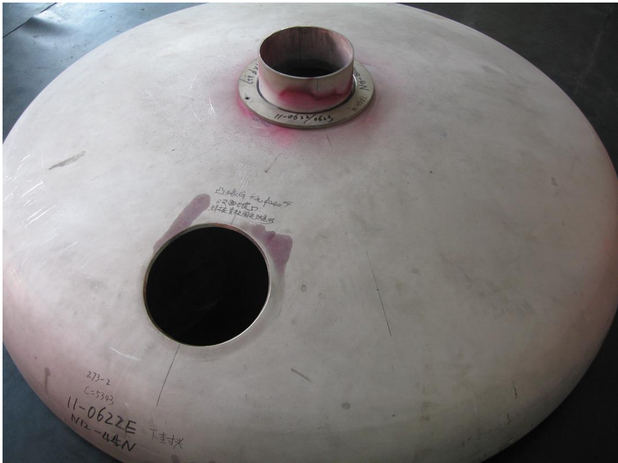
Manufacturing inspection - Weld preparation and PT tests on dish heads at Mersen Xianda (China)
