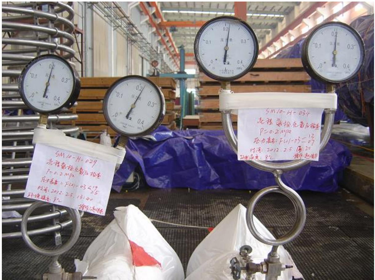
Manufacturing inspection – NH3 tests on LEP exchangers at Morimatsu Shanghai (China)
