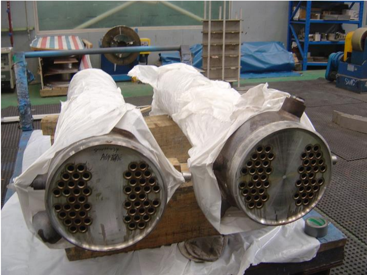
Manufacturing inspection – Check of the tube welds on tube sheets of LEP exchangers at Morimatsu (China)
