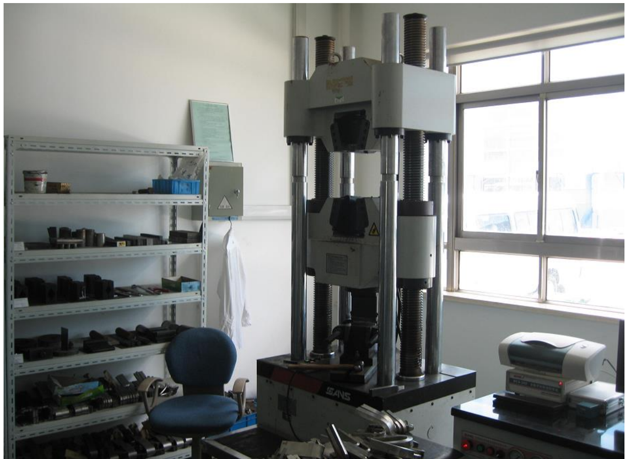
Manufacturing inspection – Witness of mechanical tests on probes at Morimatsu Shanghai (China)
