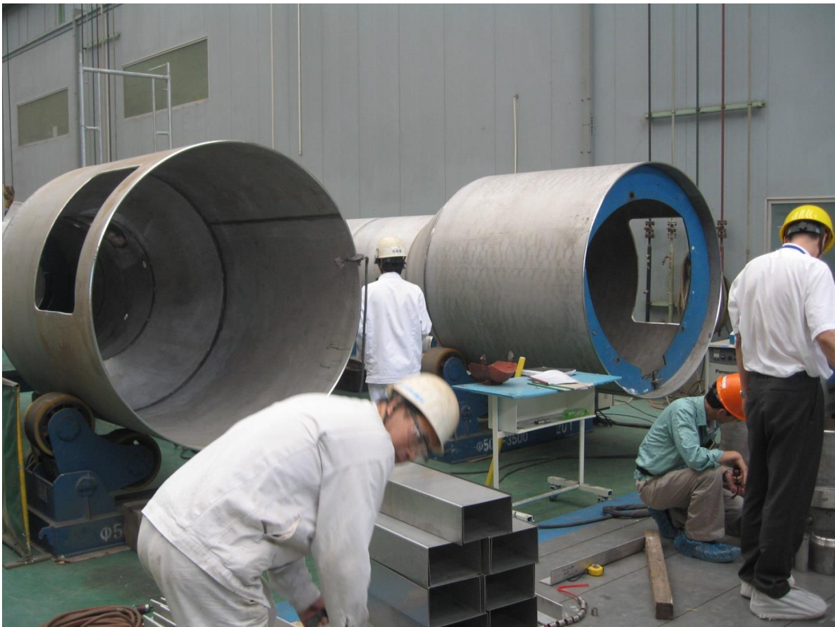
Manufacturing supervision - Shells of heat exchangers at SMPV Morimatsu Shanghai (China)
