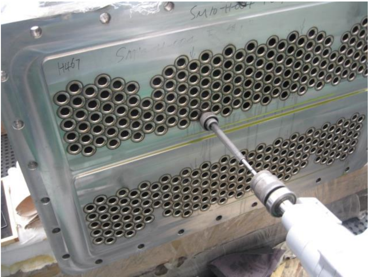
Manufacturing inspection – Check of the tube expansion of the TEP DZ exchangers at Morimatsu (China)
