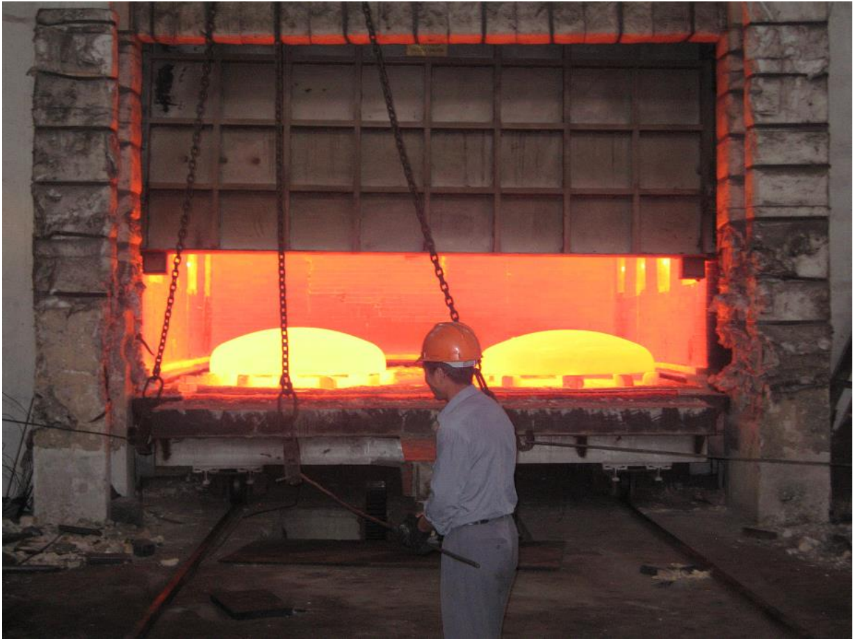
Manufacturing inspection – Check of heat treatment conditions of dish heads at Wuxi (China)
