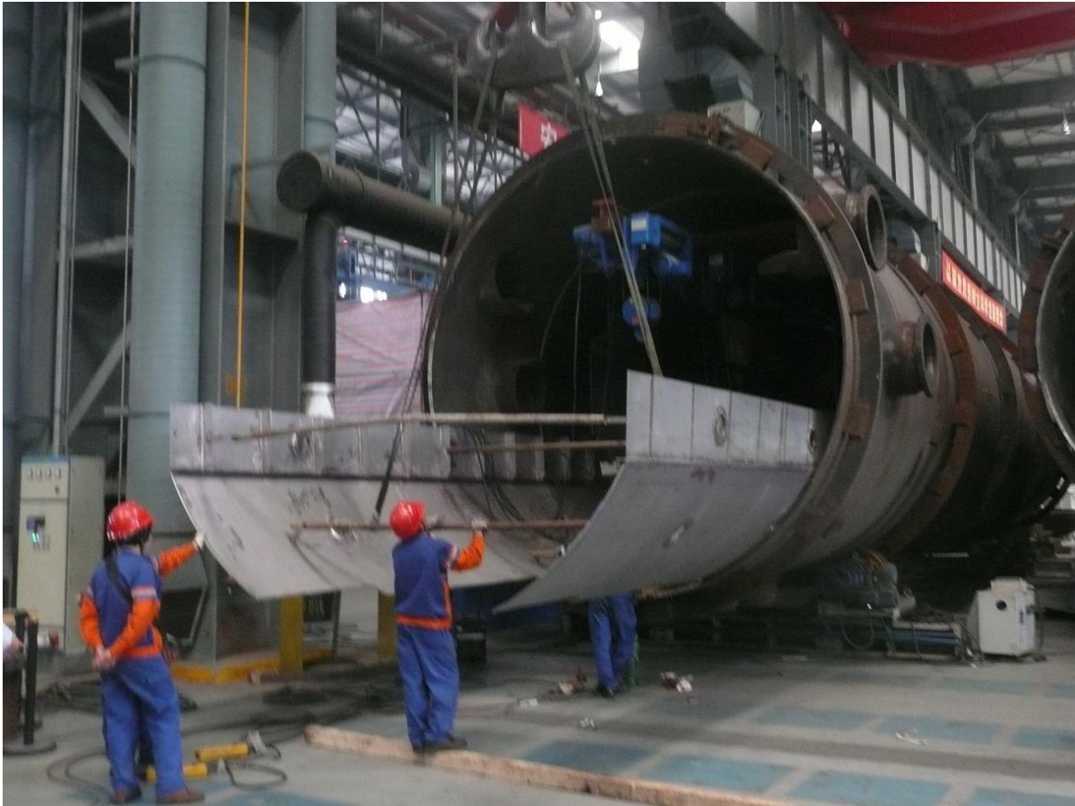
Manufacturing supervision - Moisture Separator Reheaters (MSR) at Dong Fang H.M. at Nansha (China)
