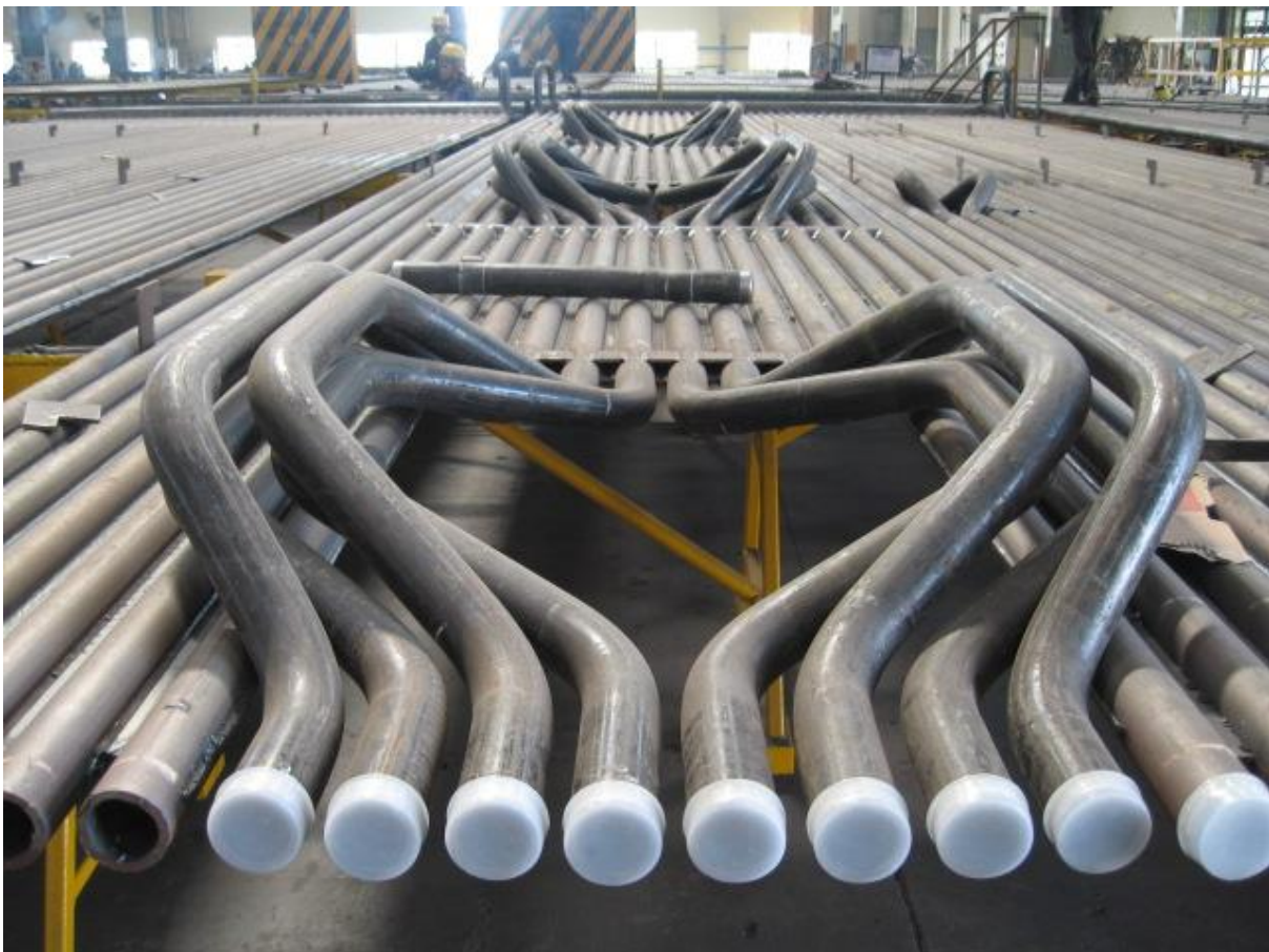
Manufacturing supervision - Boiler membrane panels openings to install burners at Thermax (India)
